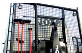
Impact tested front wall
