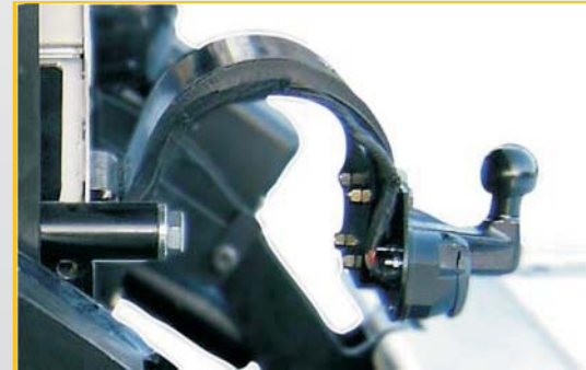
Option: Towing ball coupling, quick and easy installation, retro fittable.
